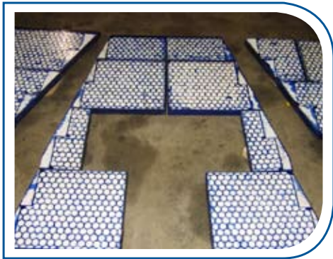
35mm Duaceramic liners for an apron feeder
