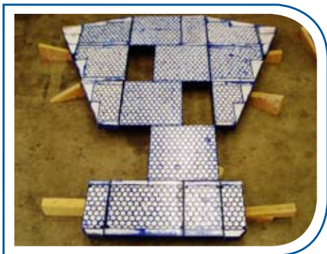
35mm thick Duaceramic liners for a ship loader
