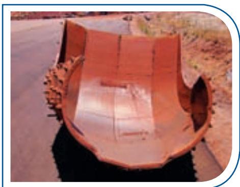
The above chute shows little signs of wear after 6 months
