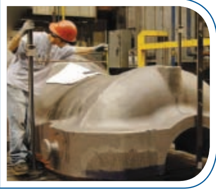
Large steel turbine housing
