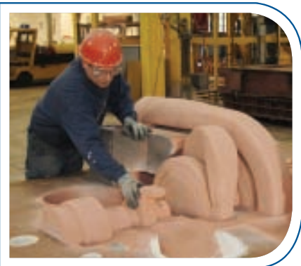
Molding/core making (complex pump housing)
