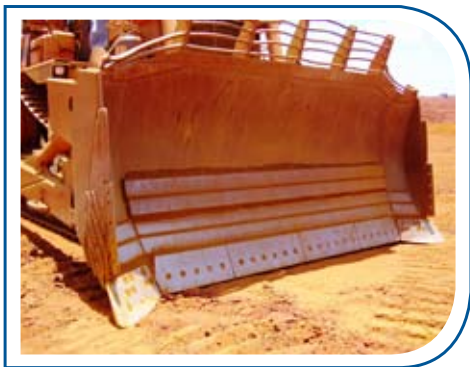
Dozer with Wearalloy tumble bars
