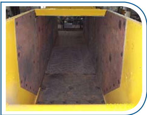
Chute lined with Wearalloy plates
