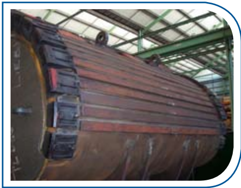
Bucket with Wearalloy strips
