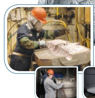
Extensive non-destructive testing including Linatron radiography for section thicknesses up to 17"/432mm
