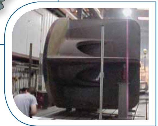
One of sixteen 32,340 lb (14,673 kg) BRADKEN® TLP Node castings for BP Thunder Horse
