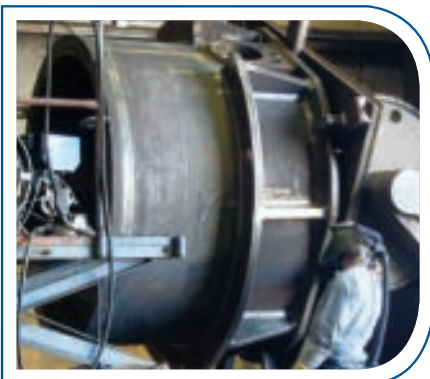
Heavy fabrications using weld positioners
