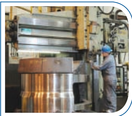
Turning/Machining (Off-shore Oil Platform Riser Basket)
