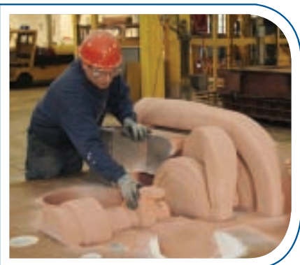
Molding/core making (complex pump housing)
