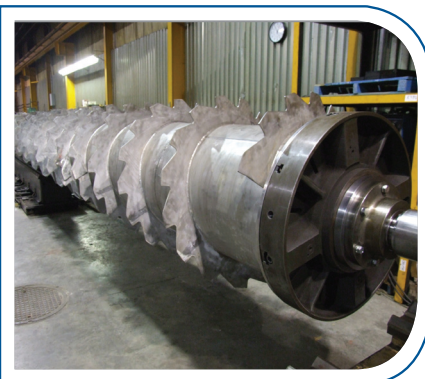
Duplex 2205 bleach screw repair
