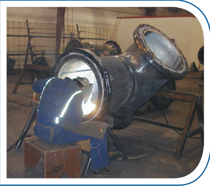
Bradken fabricates parts and pipes to be overlaid
