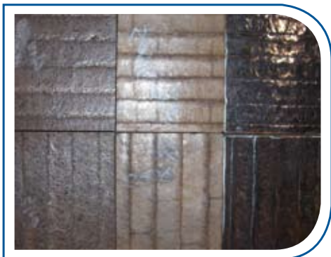
Duaplate - Standard (left), Smooth (Centre) and Polished (Right)
