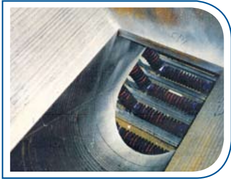
Duaplate Smooth coal conveyor feed chute
