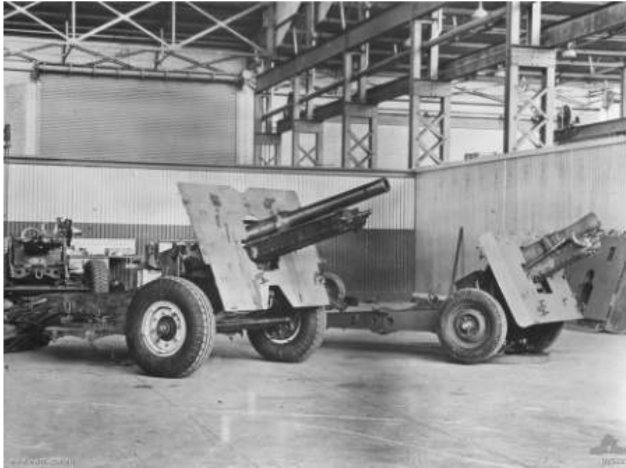
Standard 25 pounder with the first short 25 pounder (shortened barrel), produced at the works of Charles Ruwolt Pty Ltd.
